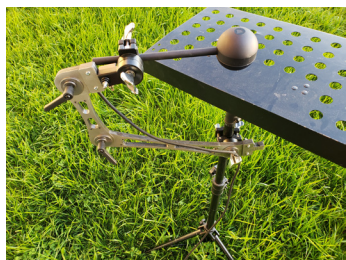
Figure 1: Pictured is a 2-segment adjustable locking arm
