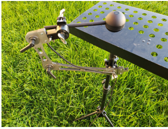
Figure 1: Pictured is a 2-segment adjustable locking arm
