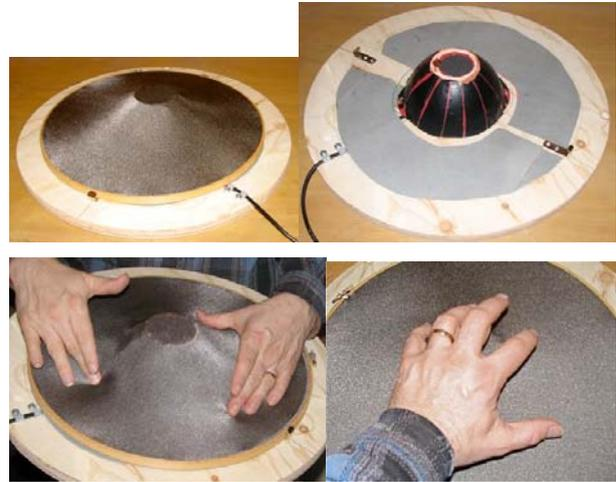
Figure 13: Tablo Fabric Multitouch Controller
