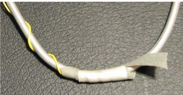
Figure 6: Bendable Pressure sensor
