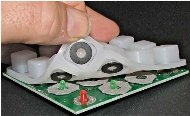
Figure 9: Pressure Sensitive Monome Adaptation
