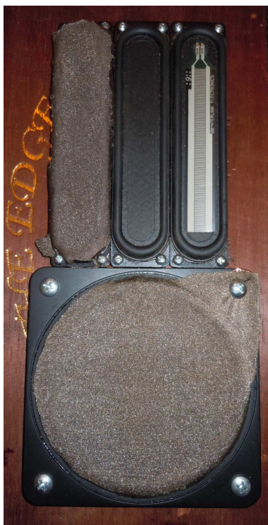
Figure 3. Haptic Speakers, fabric (top left and bottom) and commercial FSR (top right).
