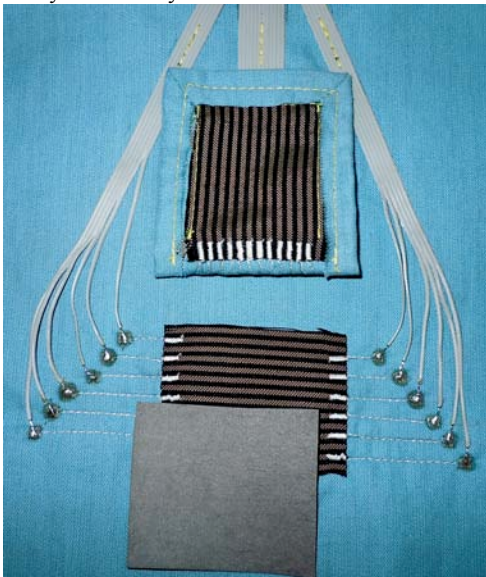
Figure 1: Strain-relieved cabling and solder pad
